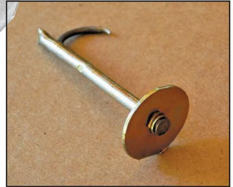
Figure 5 – Tubular with nail fastener.
