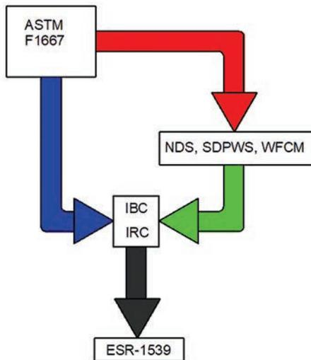
Figure 2 – Relationship between ASTM F1667, AWC Standards, the I-Codes and ESR-1539
