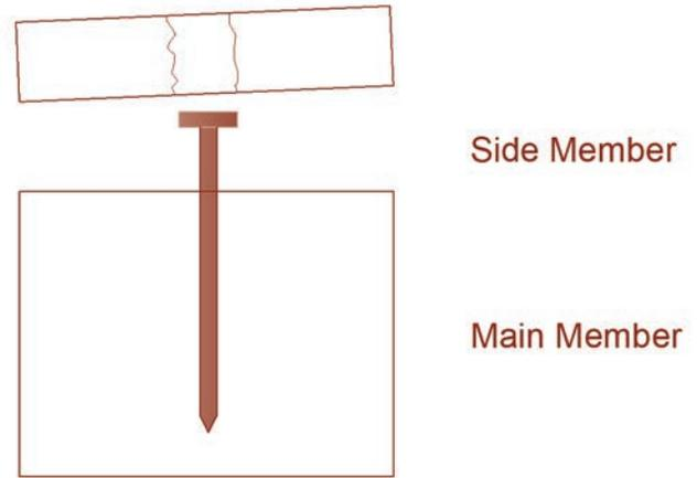
Figure 8 – Connection failure from pull-through.
