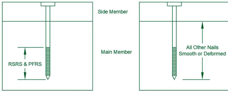
Figure 7 – Nail penetration basis for determining withdrawal.
