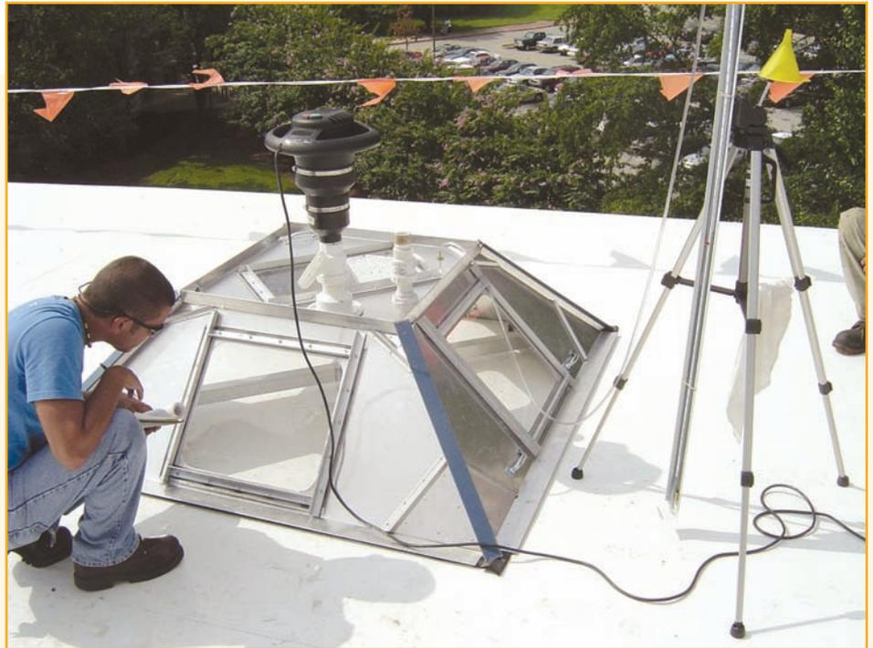
*A consultant checks a wind uplift chamber on a roof to determine the system's uplift resistance. (Photo courtesy of Roof Engineering Inc.)*
