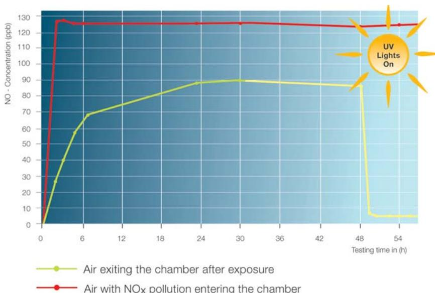
Figure Two. The Franhofer Institute set up a test cell that shows how smog-eating tile causes a significant decrease in air pollution when exposed to UV lighting. The UV rays actually encourage smog reduction with a photocatalytic action.
