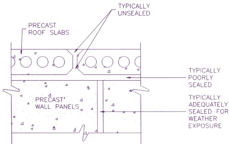
Figure 18: Freezer roof structure detail showing infiltration points.
