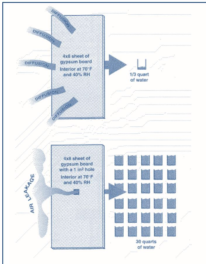
Figure 4: Moisture transport by diffusion versus air leakage.
