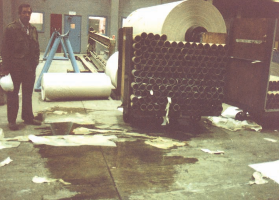
Figure 4—A plant manager knows well the cost of an interrupted manufacturing operation. A prematurely failed roof system produced widespread water entry and machine downtime in this paper mill. The warranty didn't help.
