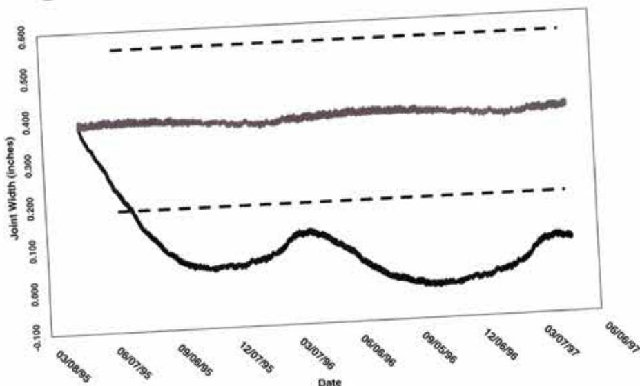
Figure 6 - The expected performance with consideration of only thermal movements as compared to the performance considering both thermal and moisture-related movements. The dashed lines represent  $\pm 50\%$  acceptable movement range.
