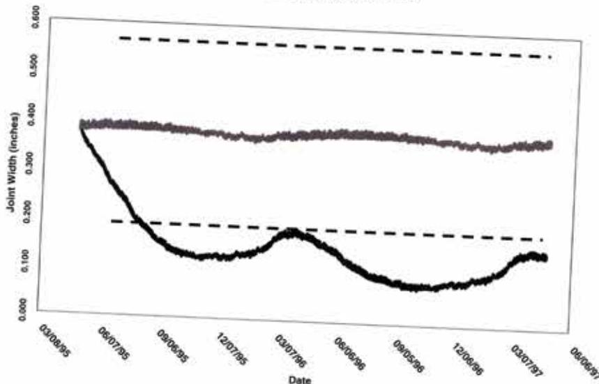
Figure 7 - Sketch showing estimated actual movement considering both thermal and moisture-related movement based on a reduced coefficient of hygroscopic expansion. The reduction of the coefficient accounts for fastening between the wall layers.
