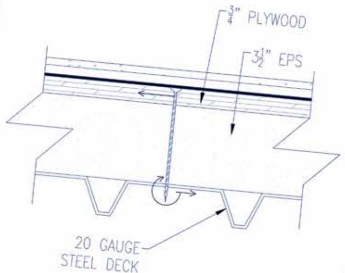
Figure 5 – Deck and fastener configurations.
