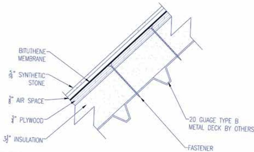
Figure 2 – Cross section of the as-designed and constructed wall/roof assembly.
