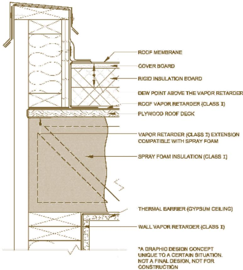
**A GENERAL RECOMMENDATION FOR A ROOF SYSTEM AND PARAPET DETAIL \***
