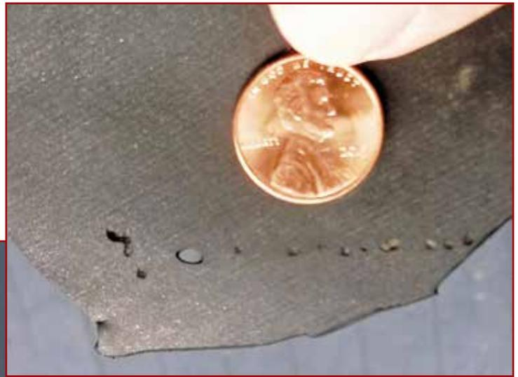
*Figure 4 – Top surface of planter liner showing tiny insect boreholes. These are unique and cannot be replicated by drill gun, ice pick, golf shoes, falling limbs, spiked hail, or any other type of mechanical contact.*
