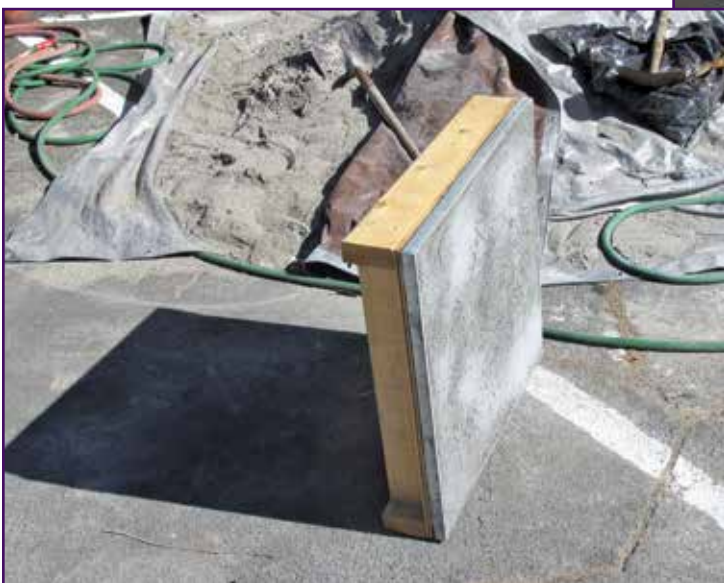
Photo 4 – Small test panels (#16 through #31) measured 2 feet square.
