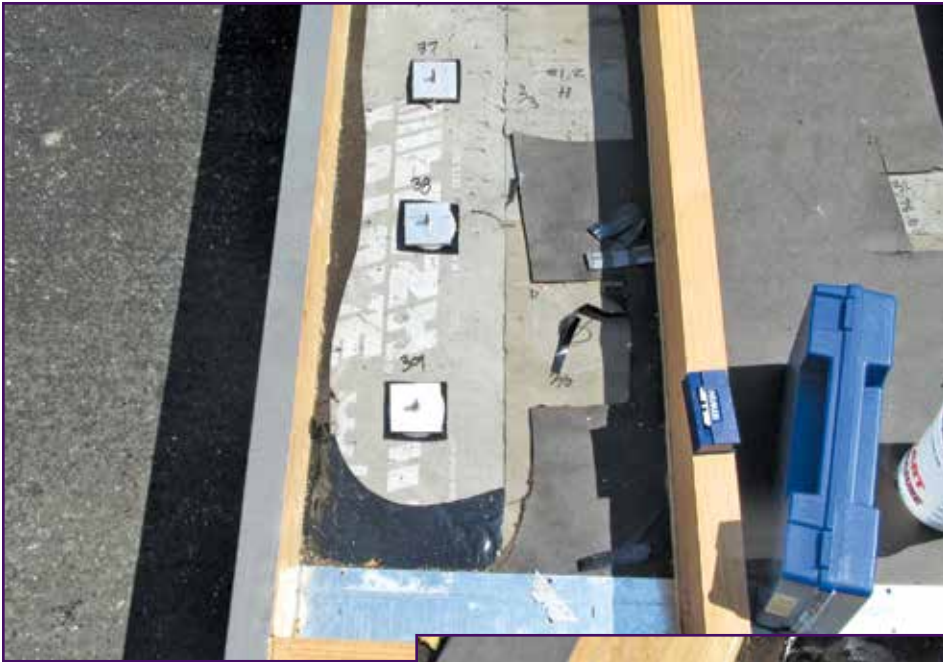
Photo 5 – Typical layout for pull-testing the 2-in. loading fixtures with Shimpo FGE force meter.
