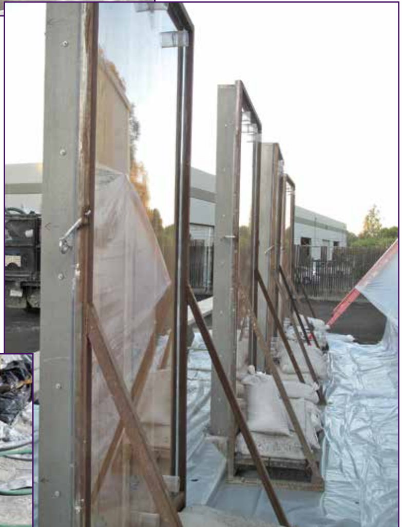
Photo 3 – Backside of testing frames with test panels in position. Note the weather-protective Plexiglas sheets (with ports that promote air flow) installed at the inside face of each mock-up wall.
