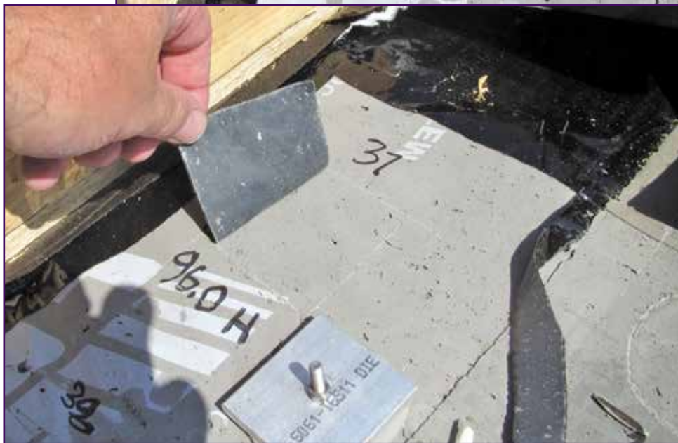
Photo 7 – At test location #37, the 2-in.-square section of the tested membrane that could not be pulled perpendicularly from the stucco easily could be peeled laterally (<2.0 lbf).
