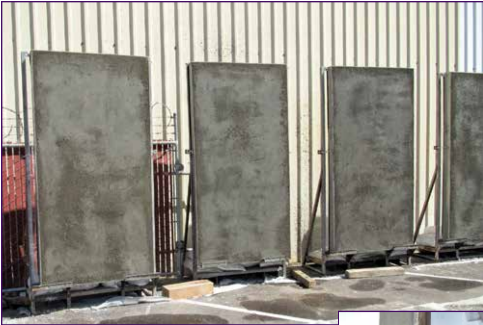
Photo 2 – These large mock-up panels (measuring 4 x 8 ft.) were lathed, scratched, and browned in July 2013. A finish coat was later applied after completion of the moist-curing process.
