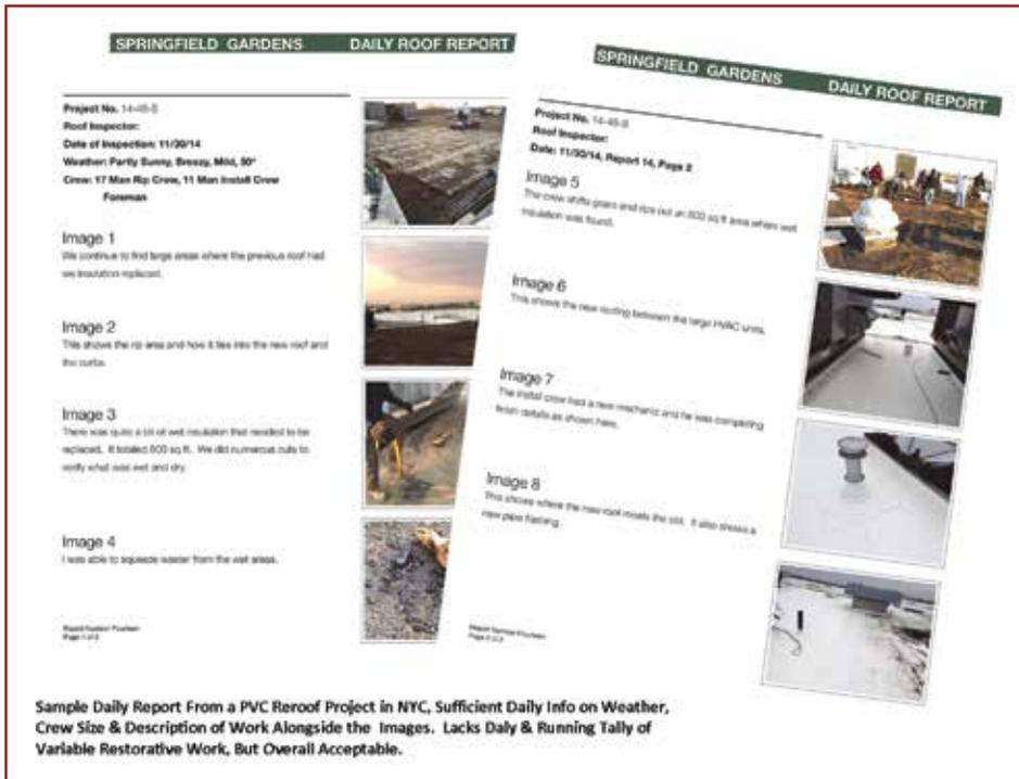
Figure 1 – Sample daily report from a PVC reroof project in New York City. Sufficient daily information on weather, crew size, and a description of work accompany the images. Lacks daily and running tally of variable restorative work, but acceptable overall.
