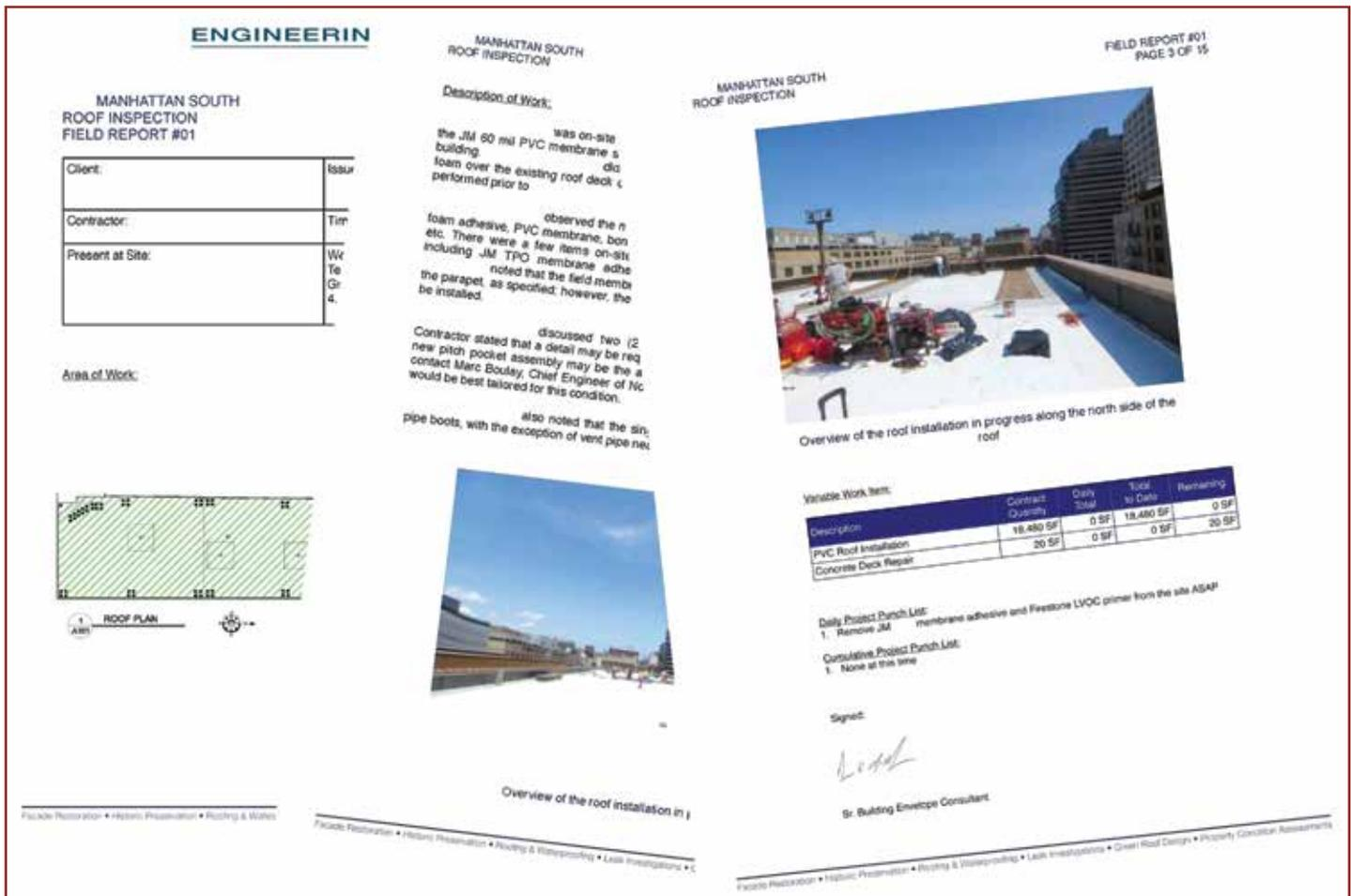
Figure 2 – A more complete report with a scaled, color-coded roof plan, text documentation, and a tally of the variable work items, as well as color images with work descriptions.
