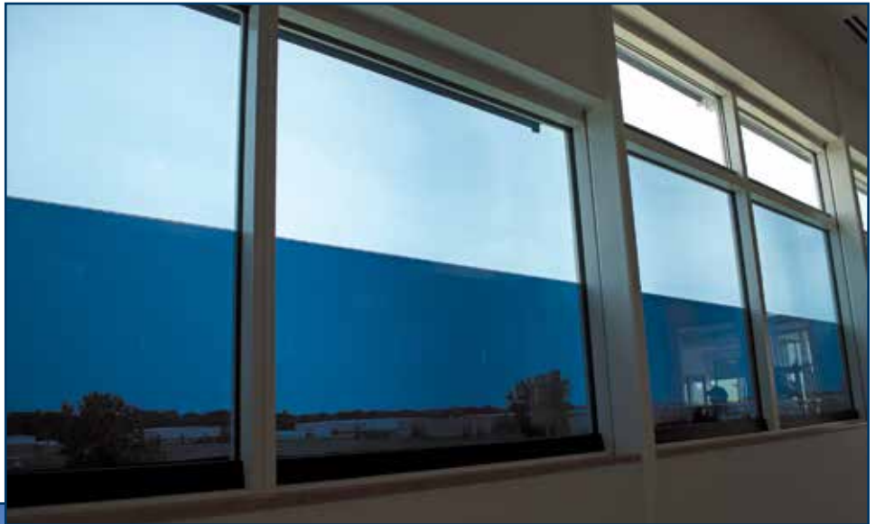
Figure 4 – An example of one of the new advances in electrochromic glazing: in-pane zoning. This feature provides the ability to optimally balance the need for glare control with adequate daylight admission, energy performance, and light color quality. Photo courtesy of SAGE Electrochromics, Inc.
