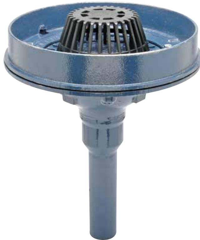
Figure 4 – A 363-mm (14½-in.) diameter siphonic overflow roof drain with standard dock. The key to the operation of a siphonic system is eliminating all air from entering the piping system. This is achieved by placing an engineered secured baffle into the base of the sump that breaks up the Coriolis Effect of rotating water.
