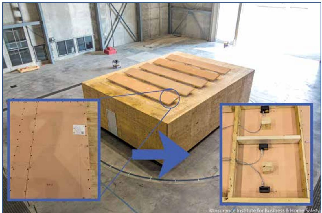
Figure 1 – Photograph of solar panels on the roof of a building in the IBHS test chamber.
