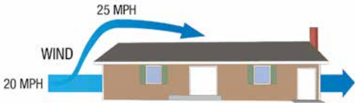
Figure 1 – During strong gusts on relatively flat roof surfaces, air pressure can drop and act as a vacuum, pulling roofing material into the air stream.
