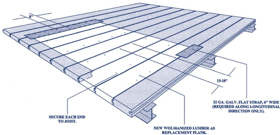
Figure 6 – Repairs are probably best made by replacement in kind, although tongue-and-groove integrity must be maintained. Any variations of the repair depicted must recognize this aspect.
